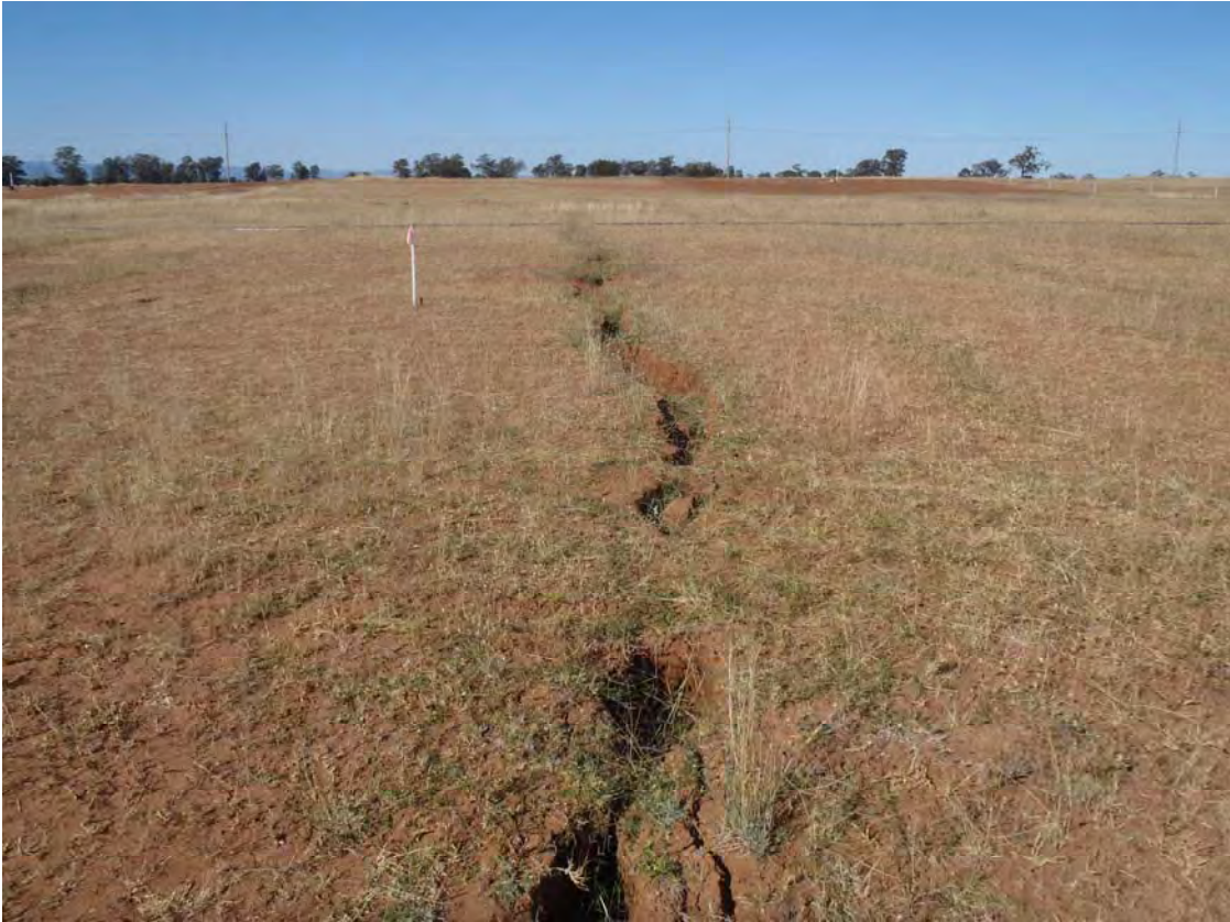
Photo 4: LW101 Surface Crack
